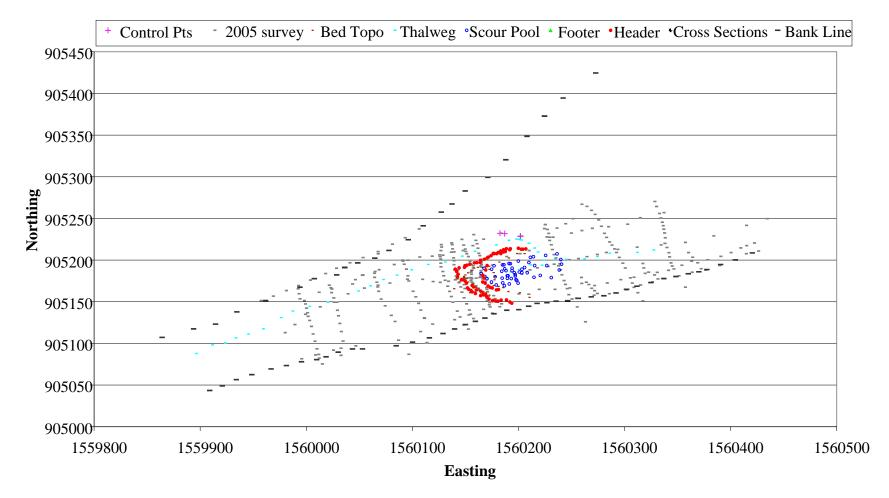
Figure 4. Survey data collected for East Fork Salmon Structure EF 7-8.
