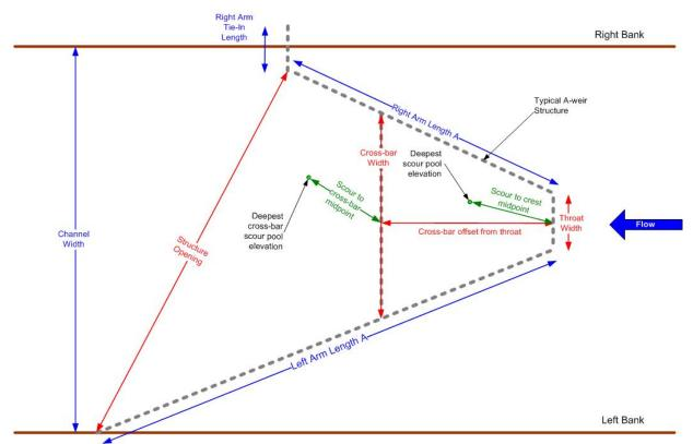
Figure 2. Plan view schematic of a typical A-weir river spanning rock structure.
