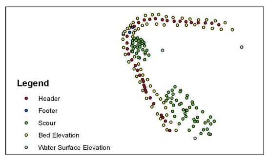
Figure 71. Survey data collected for Entiat River structure at RM 3.1.
