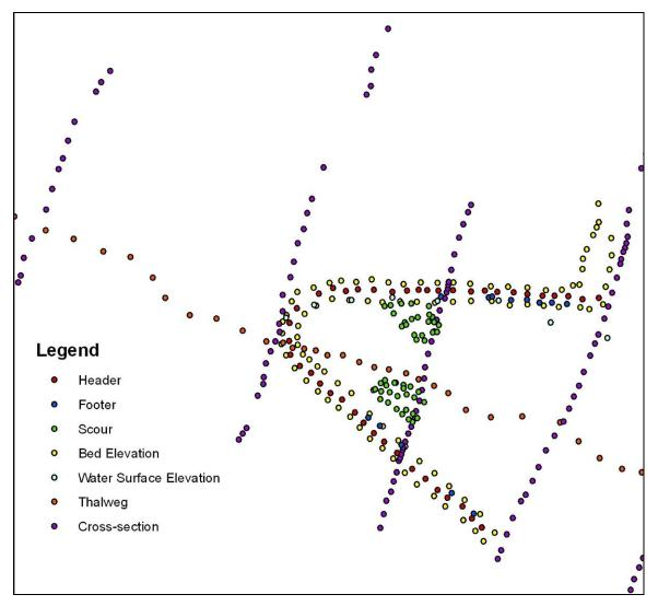
Figure 87. Survey data collected for Entiat River structure at RM 3.4.
