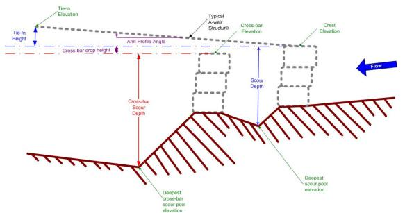
Figure 3. Profile schematic of a typical A-weir river spanning rock structure.
