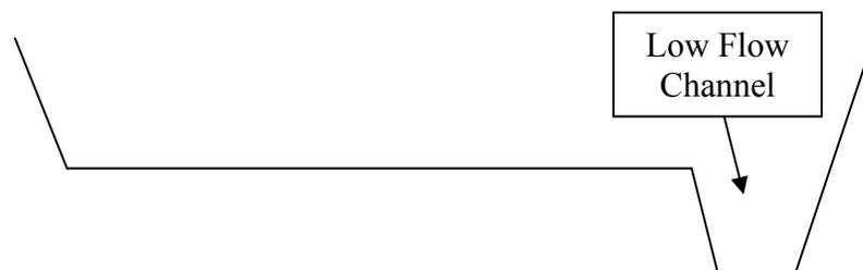
**Figure 4-3 Rock Ramp and High Flow Sill (Case B)**
