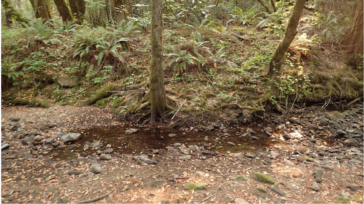
Figure 11. Upper Redwood Creek gage pool 8/27/20, flow coming into the gage pool (0.00076 cfs), but the riffle crest was dry. The sensor was not submerged, just the tip touched the water to read water level.
