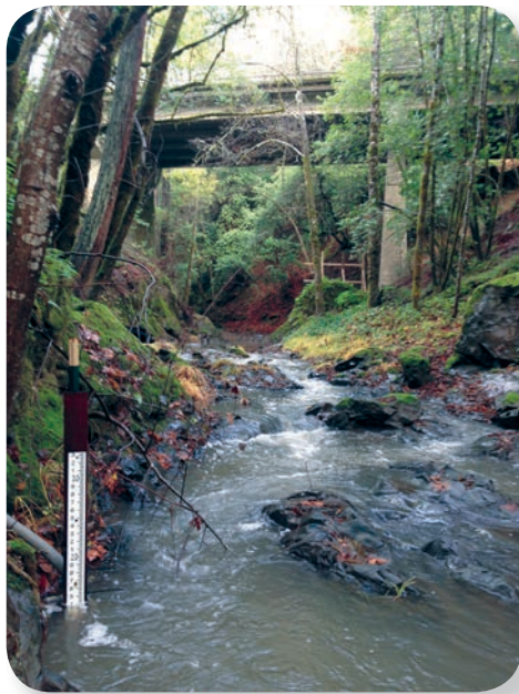
Gauging station on Indian Creek that provides data to support new environmentally beneficial wintertime diversion water rights under the North Coast Instream Flow Policy.
