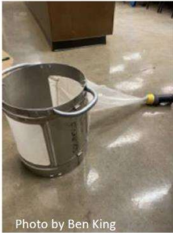
Samples collected using 0.09 m 2 hess sampler.
