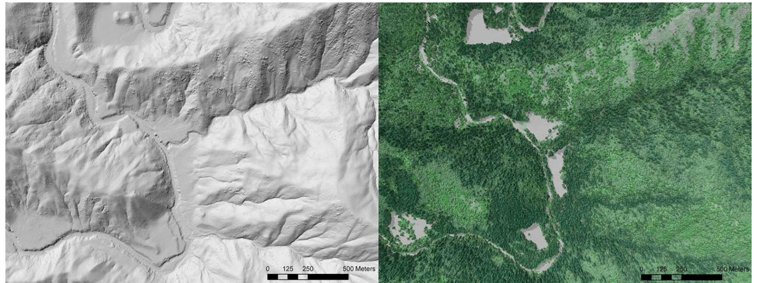
Angelo Coast Range Reserve. 2004 LiDAR. Left processed into Bare-earth DEM. Right processed into Canopy elevation and Tree height.
