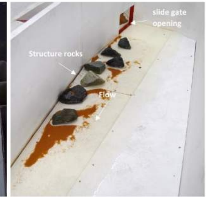
Photo 4. Deposition patterns at the fishway exit at 206 cfs (some sands).
