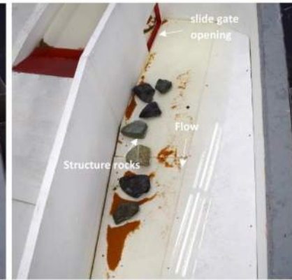
Photo 3. Deposition patterns at the fishway exit at 115 cfs (some sands).
