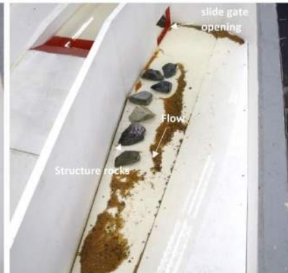
Photo 6. Deposition patterns at the fishway exit at 850 cfs (fine gravels with some coarse gravels).
