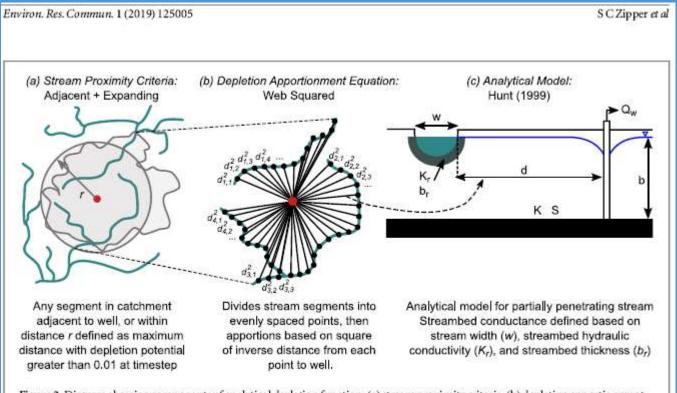
Figure 2. Diagram showing components of analytical depletion function: (a) stream proximity criteria, (b) depletion apportionment equations, and (c) analytical model.
