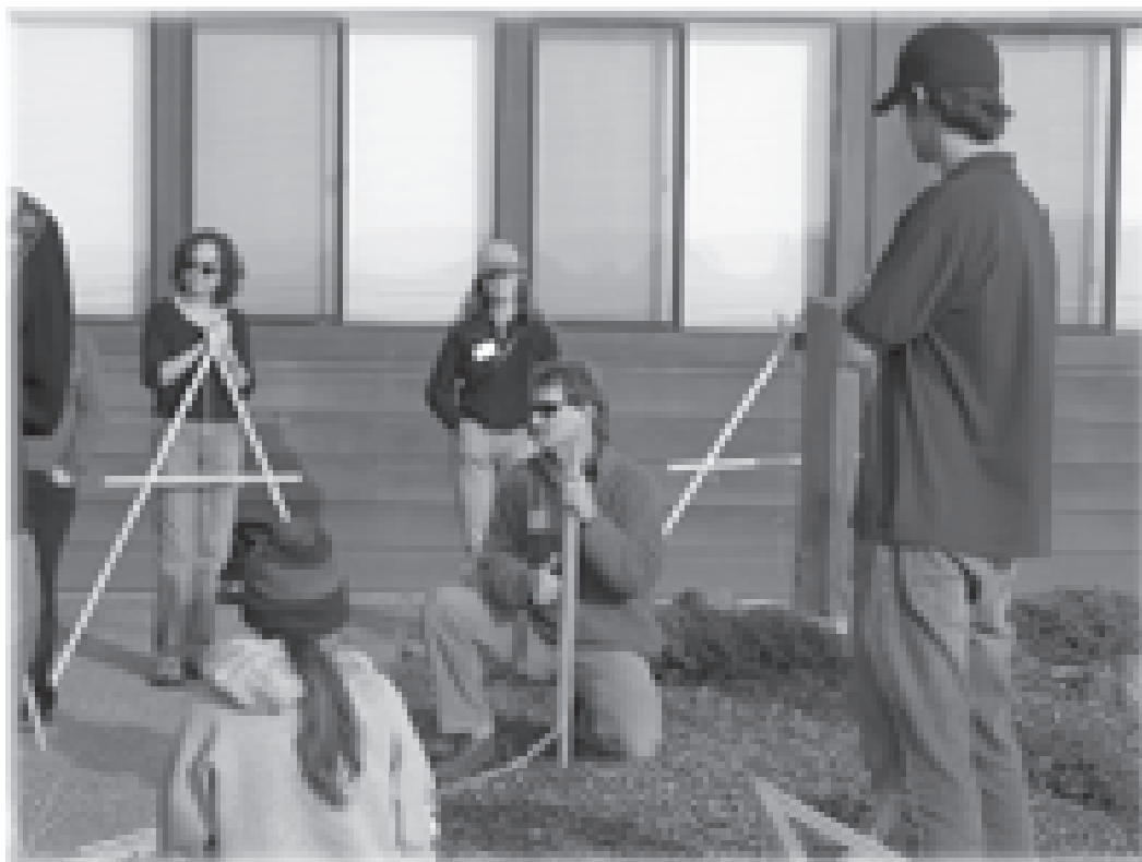
Brock Dolman demonstrating the construction of a simple A-Frame used for finding and marking a level contour line on a slope for rainwater harvesting projects.
