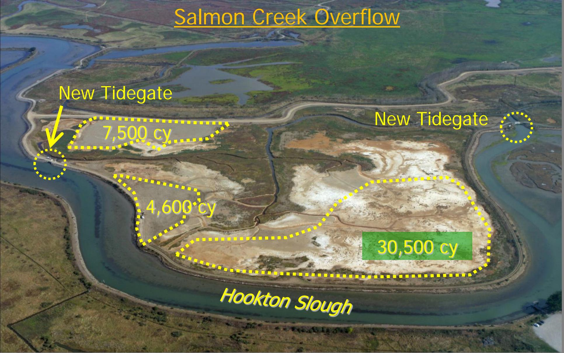
Spoils from channel excavation used to raise subsided land and restore salt marsh.
