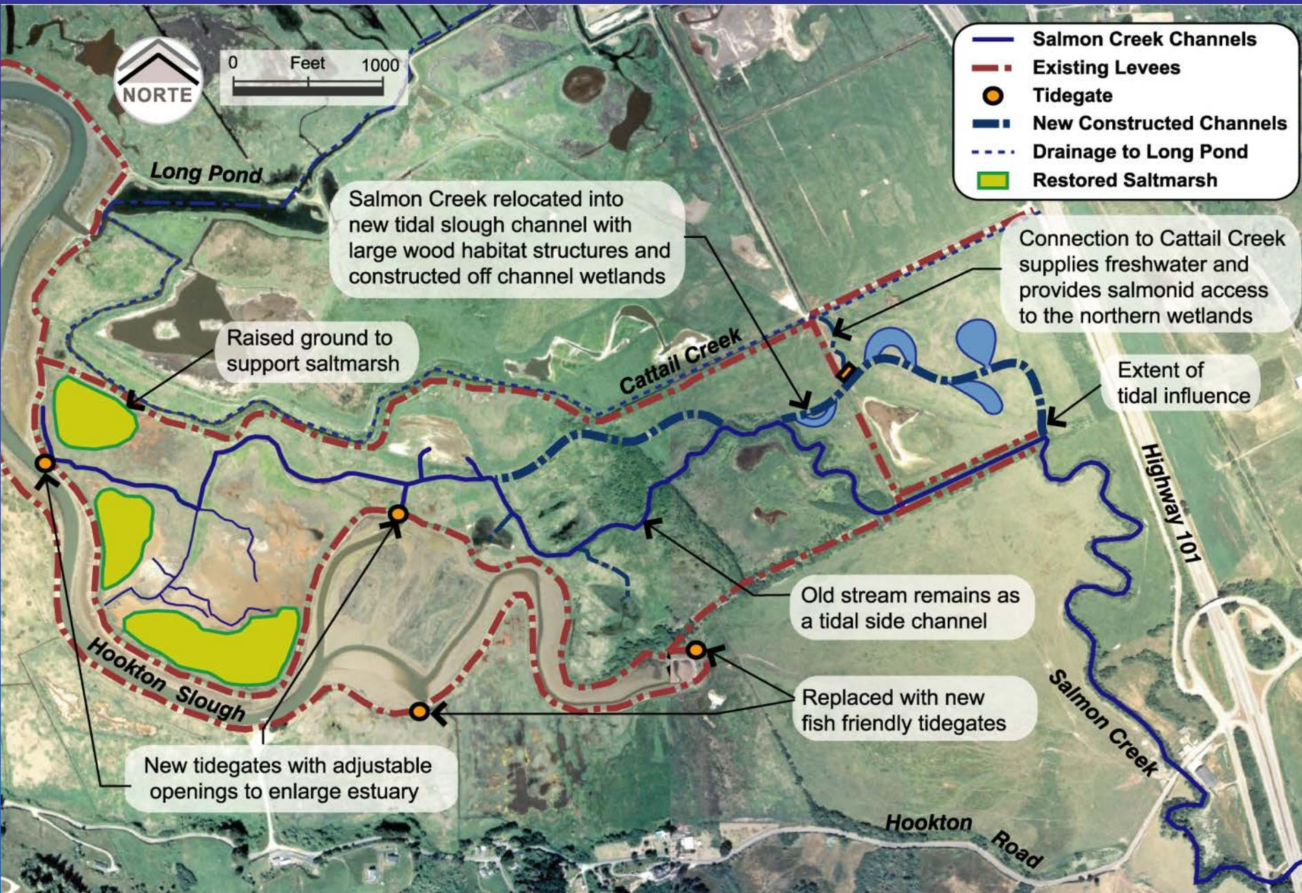
Salmon Creek relocated into new tidal slough channel with large wood habitat structures and constructed off channel wetlands
