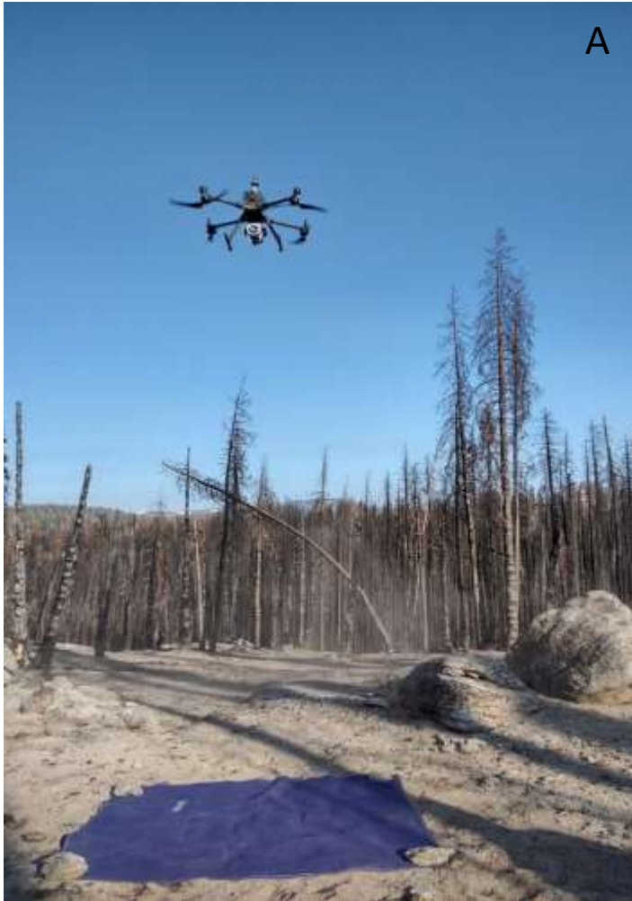
A. GTAC Drone collecting LiDAR at Southern Sierra partner site Lower Grouse Meadow B. Middle Creek Meadow Hillshade
