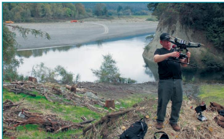
*Preparing a UAV for deployment as part of a road decommissioning/Fish barrier removal project. The use of UAV's and photogrammetric techniques is becoming a popular tool for environmental restorationists. photo by Tom Leroy*
