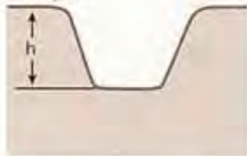
Class II. Channelized h < h_c floodplain
