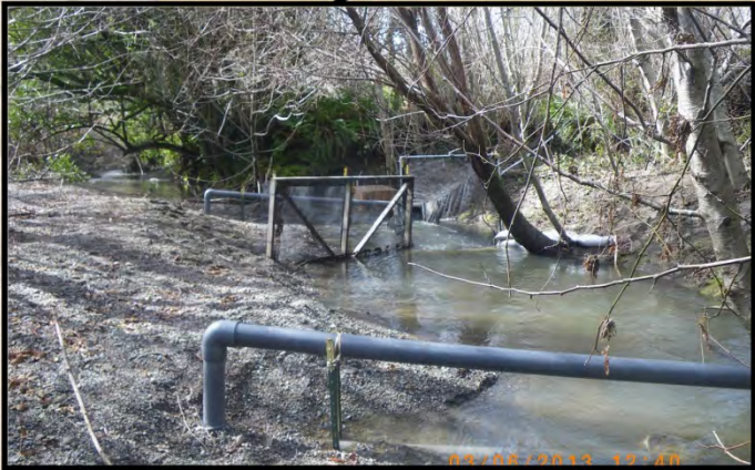
Upper antenna array and smolt trap, Rkm 3.70
