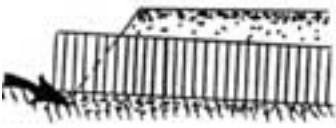
d) Outlet too high, resulting in shotgun culverts and much erosion, releasing sediment into nearby creeks
