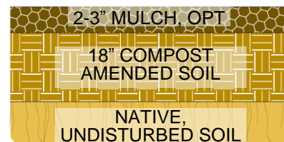
Figure 1 To ensure proper water quality treatment, an 18" layer of healthy soil is needed in all bioretention facilities.
