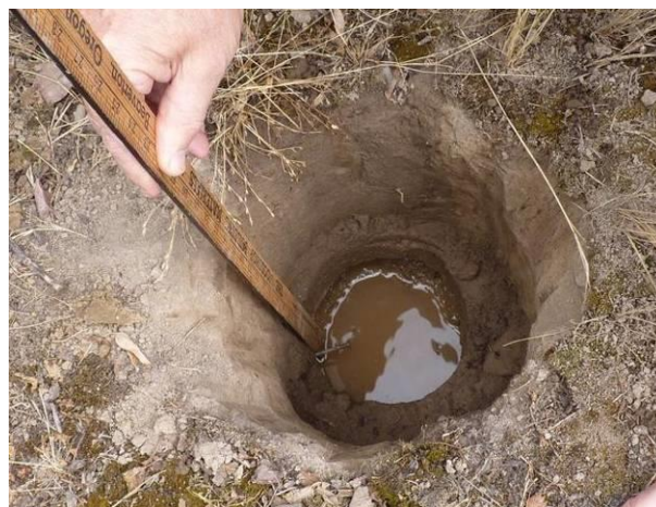
Figure 3 A shovel was used to dig most of the way then a 6" diameter post hole digger was used to reach the proposed bottom elevation of a rain garden. Measure the drop in water from a known, stable marker.
