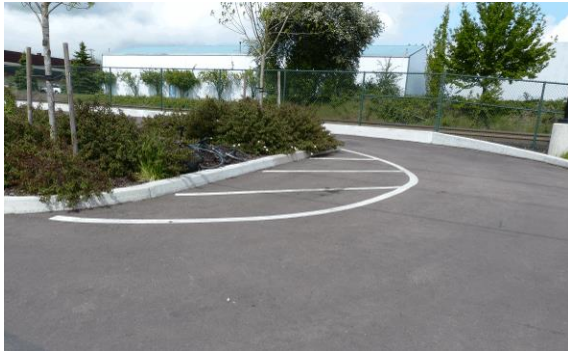
Figure 8. Many small unused pavement areas add up to a lot of unnecessary pavement in a watershed.
