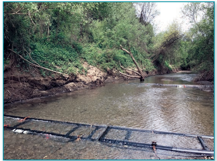
Dual PIT antenna array on Porter Creek Photo Credit: California Sea Grant
