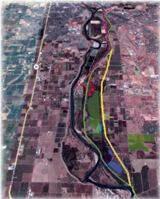
Oblique satellite view of levee setback alignment and conceptual floodplain connectivity project; lower Feather River, Yuba and Sutter Counties, CA
